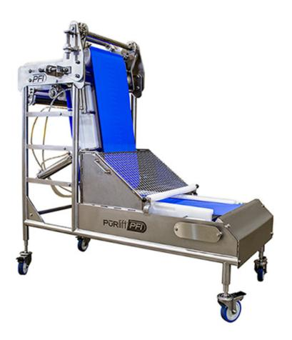
The PURlift positive drive vertical lift conveyor fits in tight spaces where you need to elevate your food processing line. Its positive drive system and self-tracking belt keep your product and operation moving. Sanitation is more efficient with caster footing to move on and off the line quickly, and a pneumatic belt tensioning system doubles as a quick release take up.
