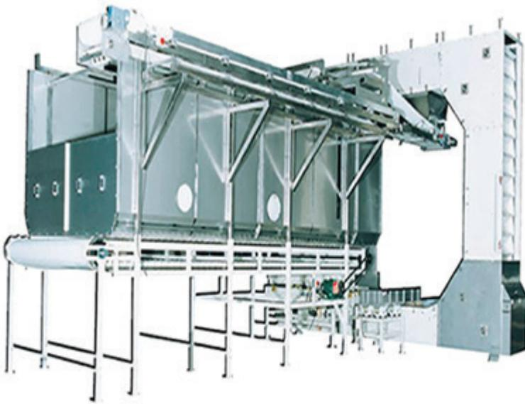
The Storeveyor allows processors to more efficiently store and feed product throughout food processing lines. It temporarily accumulates and stores large volumes of product in a stainless steel bin, then uses belt conveyors to discharge it to the next process. It can be integrated with a range of infeed and outfeed options, including elevators, vibratory feeders, and more.
