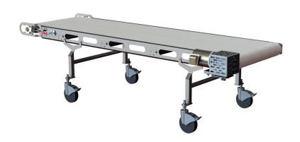
Horizontal Belt Conveyors are common conveying solutions to move product throughout your food processing plant. It's flexible, with customizations to fit your line and options to optimize sanitation, product handling, and performance. Its flat-bed stainless steel frame and tool-less belt removal allow for quick, yet thorough cleaning to keep your line moving.
