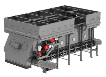
The Storeveyor allows processors to more efficiently store and feed product throughout food processing lines. It temporarily accumulates and stores large volumes of product in a stainless steel bin, then uses belt conveyors to discharge it to the next process. It can be integrated with a range of infeed and outfeed options, including elevators, vibratory feeders, and more.
